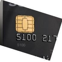
This microchip as well as the magnetic stripe on the back of cards should make it nearly impossible to create a counterfeit EMV card that can be used at point-of-sale terminals successfully.
